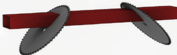
Tilting 45° inward for both heads
